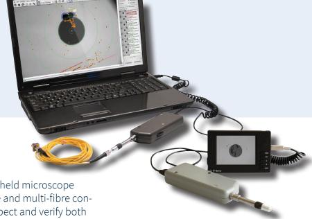
Sumix designs and manufactures handheld microscope probes for end face inspection of single and multi-fibre connectors. The probes can be used to inspect and verify both exposed connector ferrules and also through bulkhead or adapters. Suitable for both PC and APC connector types with both digital and analogue versions available.
