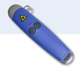
Visual fault locators (VFL) serve as a simple tool to accurately detect the location of faults along a fibre optic cable. This compact pocket sized unit injects visible light into the fibre strand. Any breaks, microbends or faulty cable will display a visible red light to indicate the problem area.
